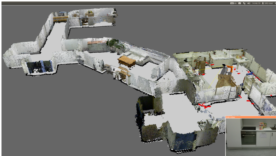
Fig. 1. User interface in zoomed-out perspective with apartment-sized environment mapped using voxel-based mapping technique
